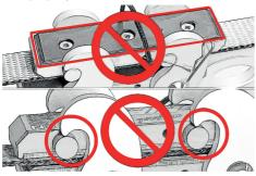
Ensure parallel alignment with the slackline!
