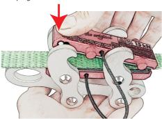
2. Push the clamping plate forward, until a click sound confirms locking, and the pegs latch into the hooks. The plate is now secured against inadvertent unlatching, and the lineGrip is ready to use.
