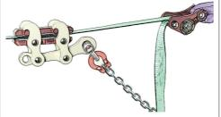
5. When the tensioning device is fully contracted, remove all slack between the lineGrip and the web lock (as tight as possible). Then **slowly** release the tensioning device so the load of the system is transferred gently onto the webbing locker.
