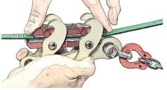
2. Attach the lineGrip preferably first to the webbing and then to the tensioning device to facilitate an untwisted connection (make sure that the rope or chain is not twisted).
