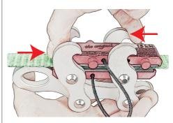
2. Remove the loose plate by lifting up the front end with the spring balls first, then retrieve the plate in a backwards and upwards motion.
