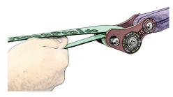
1. Attach the slackline to the anchor points by means of appropriate anchor/fixation devices (web locks), and pretension by hand as well as you can easily handle (we've compiled some pretensioning tips and tricks on <a href="https://www.linegrip.com/pre">www.linegrip.com/pre</a>;-)
