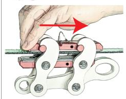
Warning: If no retainer pin is installed, the lineGrip may fall off the webbing due to a shaking or oscillating slackline, when no load is applied to the load eye of the load bracket.
