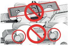
Ensure parallel alignment with the slackline!
