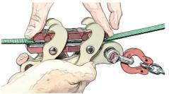
2. Attach the lineGrip preferably first to the webbing and then to the tensioning device to facilitate an untwisted connection (make sure that the ropes or chain is not twisted).
