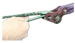
1. Attach the slackline to the anchor points by means of appropriate anchor/fixation devices (web locks), and pretension by hand as well as you can easily handle (we've compiled some pretensioning tips and tricks on <a href="https://www.linegrip.com/pre">www.linegrip.com/pre</a>;-)
