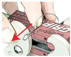
**Note:** When using the lineGrip UPSIDE DOWN, always insert the retainer pin! In this orientation, and without installed pin, it can easily fall off even a calm and steady slackline while unloaded.
