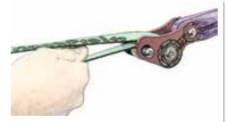
1. Attach the slackline to the anchor points by means of appropriate anchor/fixation devices (web locks), and pretension by hand as well as you can easily handle (we've compiled some pretensioning tips and tricks on <u>www.linegrip.com/pre</u>;-)
