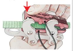
2. Push the clamping plate forward, until a click sound confirms locking, and the pegs latch into the hooks. The plate is now secured against inadvertent unlatching, and the lineGrip is ready to use.
