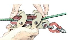
2. Attach the lineGrip preferably first to the webbing and then to the tensioning device to facilitate an untwisted connection (make sure that the ropes or chain is not twisted).
