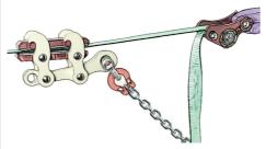
5. When the tensioning device is fully contracted, remove all slack between the lineGrip and the web lock (as tight as possible). Then slowly release the tensioning device so the load of the system is transferred gently onto the webbing locker.
