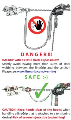
**SLIPPING HAZARD WARNING** The lineGrip must always be backed up with an appropriate fixation device while loaded! Sudden slippage can never be excluded entirely, because the lineGrip only establishes a temporary friction based connection to the webbing!
