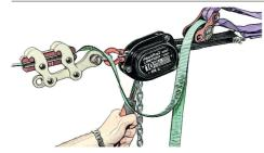
4. Now tension the slackline. While tensioning, remember to frequently(!) haul in the slack webbing between the lineGrip and the anchor! Failing to do so greatly increases the risk of damage or injury in case of slippage (see next page).
