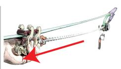
3. Unlock the tensioning device, and move the lineGrip away from the anchor as far as possible, until the tensioning device is fully extended. **CAUTION! Keep hands clear of the hooks when** releasing the load bracket! RISK OF INJURY!!!
